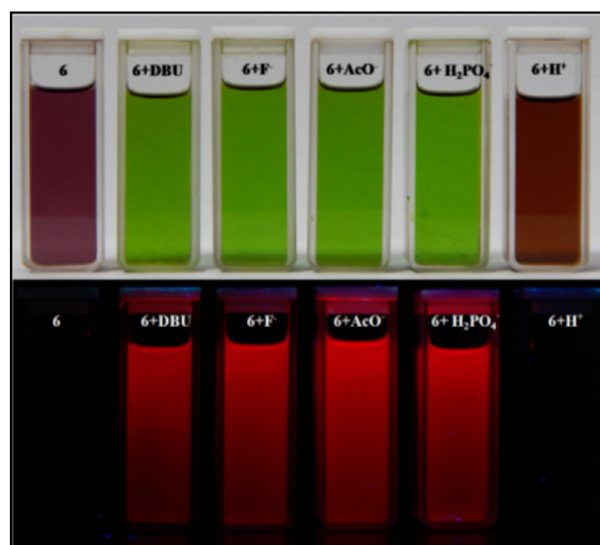
Figure 11. Colorimetric change of 6 , above under daylight and below under UV light. Picture was taken with 10 equiv additions of DBU, \text{F}^- , \text{AcO}^- , \text{H}_2\text{PO}_4^- , and TFA in \text{CH}_2\text{Cl}_2 solution of 6 ( \sim 10^{-4} M).
